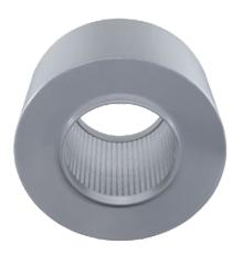
beck silencers are designed for effective use in ventilation systems. Various thermoplastic materials, such as PVC, PVC-UV, PP, PPs, PPs-el and PE, are available for both the outer pipe and the perforated inner pipe. These are particularly suitable for chemically contaminated exhaust air.
